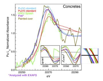
Fig. 2. XANES of three concrete samples with Pu(IV) and Pu(VI) standards. Insets show first derivative (peak position) (lower left) and second-derivative (inflection point) with magnification of zero-crossing (lower right).
