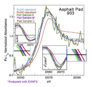
Fig. 1. XANES of three pad 903 soil samples with Pu(IV) and Pu(VI) standards. Insets show first derivative (peak position) with magnification of zero-crossing (left) and second-derivative (inflection point) with magnification of zerocrossing (lower right).
