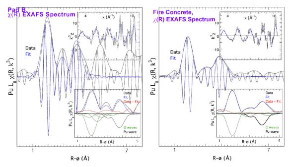
Fig. 3. EXAFS of Pad 903 soil sample B and fire-deposition concrete sample. The insets show the  $\chi(k)$  representation (upper) and the components of the fit (lower), including the difference between the data and the fit (red) and (inverted) the moduli of the individual Pu–O (green) and Pu–Pu (black) contributions.
